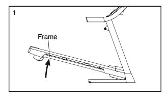
Hold the frame firmly with your right hand. Pull the latch knob to the left and hold it. Raise the frame until the latch plate is aligned with the latch pin. Then, slowly release the latch knob; make sure that the latch pin is resting on the latch plate.
